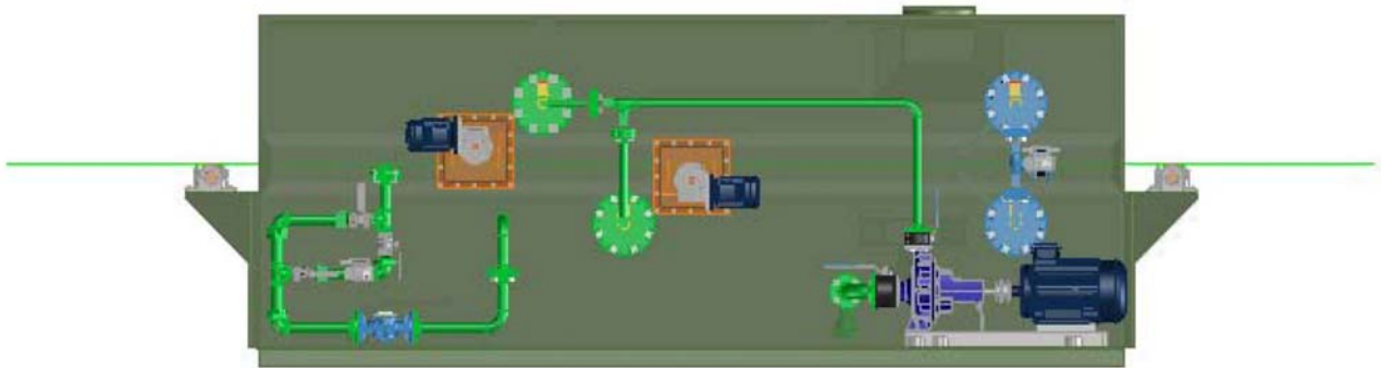
Longitudinal view of a washing machine with wet brushing system with detergent recirculation and drying system.
